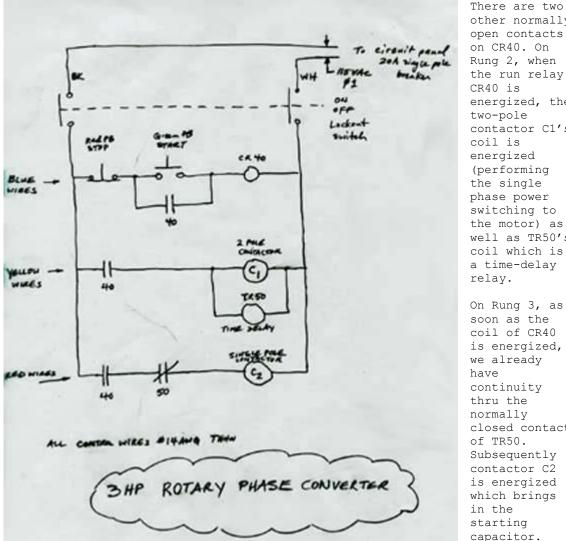
other normally open contacts on CR40. On Rung 2, when the run relay CR40 is energized, the two-pole contactor Cl's coil is energized (performing the single phase power switching to the motor) as well as TR50's coil which is a time-delay relay. On Rung 3, as soon as the coil of CR40 is energized, we already continuity
